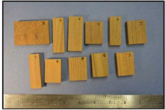
Figure 4.28. Samples after preparation for specific gravity testing.
