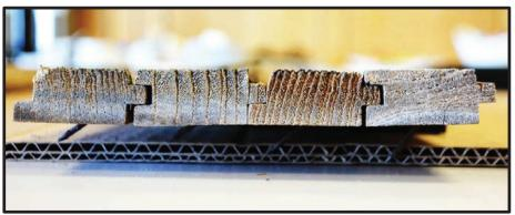
**Figure 5.11.** End grain of tongue-and-groove slats from panel that fell during a January 2014 storm. Note the loss of the upper groove rail on the slat, second from right.
