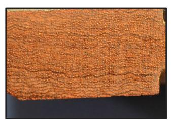
Figure 4.18. Indistinct growth rings, specimen B, end grain.
