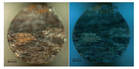
Figure 24. Sample 42 from NO6H, surface area under visible (left) and UV illumination.
