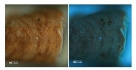
Figure 25. Sample 43 from NO6H, cross sectional view under visible (left) and UV illumination.
