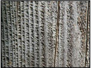
**Figure 2.1.** Example of an uncoated wood substrate with natural erosion of the lowerdensity earlywood due to weathering.
