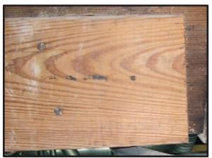
**Figure 4.19.** Flat-sawn softwood board with typical U-shaped grain pattern (material not from the Salk).
