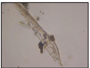
Figure 4.6. Biological growth on a wood fiber, 400x magnification.
