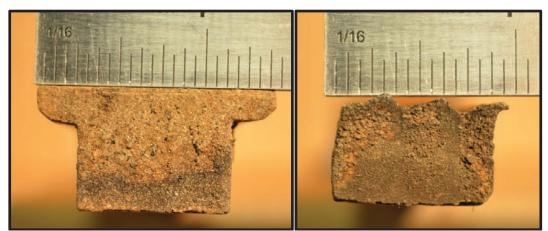
**Figure 3.9.** (Left) Specimen C, top end grain prior to sanding; (right) Specimen C, bottom end grain prior to sanding.
