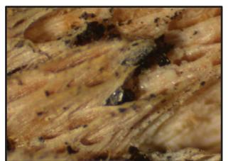
**Figure 4.2.** Specimen F showing a particle of sand and biological growth on the weathered surface.
